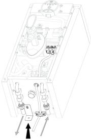
Vent & 4th fixing Cold water overflow inlet
